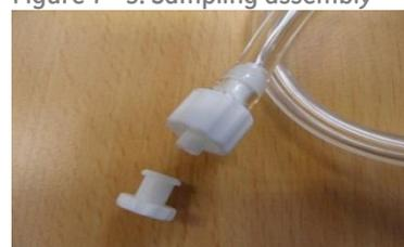
Figure 7—4: Luer fitting on assembly
