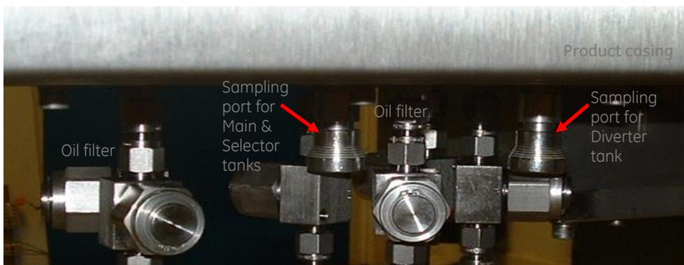
Figure 7—1: Oil filters and sampling ports (front view)
