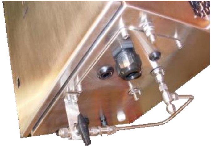
Figure 7–2: Product fitted with manual sampling arrangement
